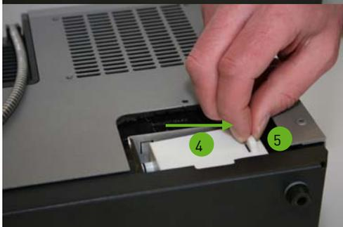
6. Push filter 4 to the right along flap 5 until the filter is exposed
