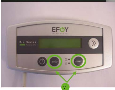
12. Press "Auto" and "Reset" together on remote control unit 7 to confirm that the filter has been changed.
