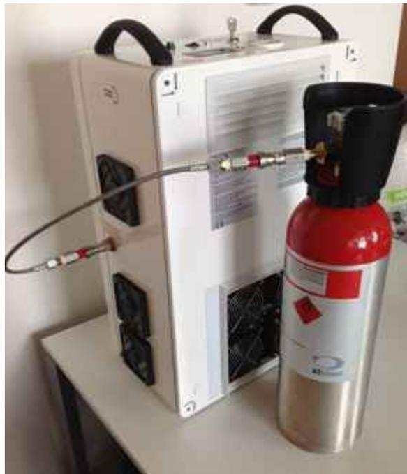
4. Turn off the device and close the black knob on the valve by turning it clockwise.
